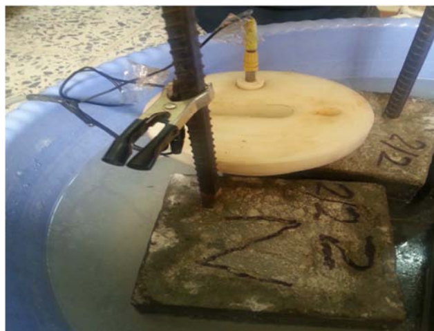
Figure 2. Concrete sample connecting with Tafel tester.
